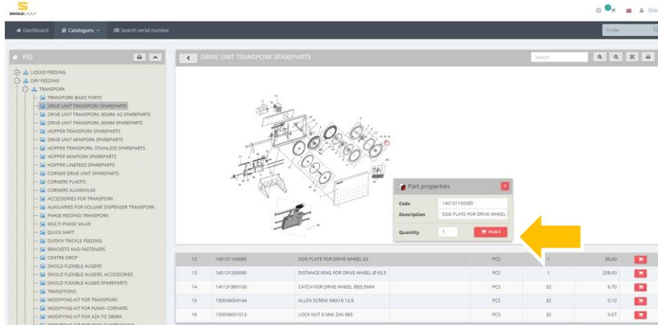
The screenshot shows the SKIOLD PARTS website interface. On the left is a navigation menu with categories like LIQUID FEEDING, DRY FEEDING, and TRANSPORK. The main area displays a technical drawing of a drive unit transpork sparepart. A 'Part properties' popup is open over the drawing, showing details for item 14013110085: 'SIDE PLATE FOR DRIVE WHEEL'. Below the drawing is a table listing various spareparts.
